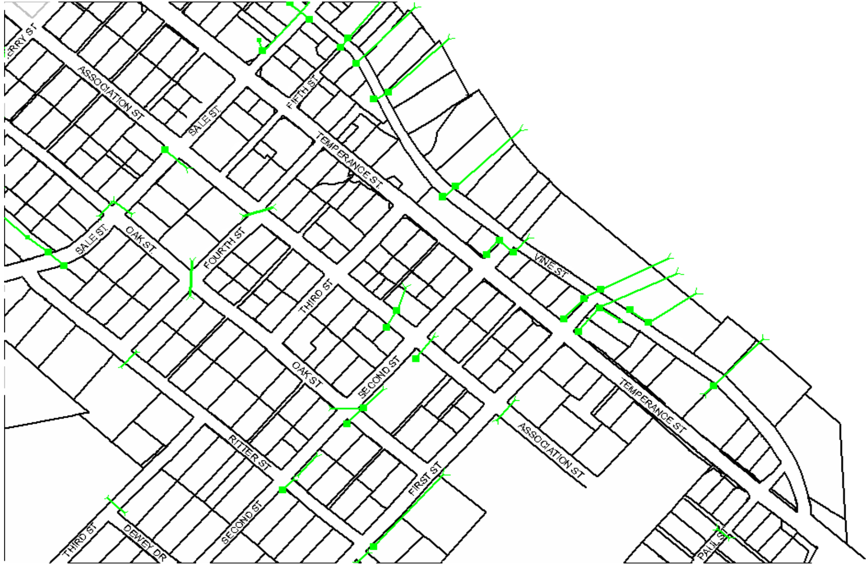
In Town #2 Storm Water System
